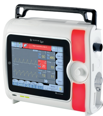
Visible alarm lights
